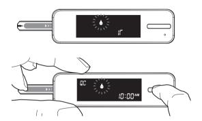
When the "appears on the display, press the Main button and "QC" will appear on the display. When the "QC" sign is displayed, the meter will not store your test result in the memory. If you decide not to perform a control solution test, press the Main button again and the "QC" sign will disappear.
