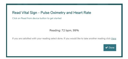
If the oximeter does not connect to the tablet, you can choose to manually enter your reading on the initial screen. Touch **Here** above the **Done** button, to return to the main screen.
